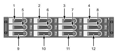
Install all of the drive carriers into the VTrak enclosure to ensure proper airflow, even if you do not populate all the carriers with disk drives.
